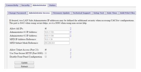
These settings allow the admin to provide additional security by limiting CACStar admin access to specified IP addresses. If the Allow all IPs box is checked, an admin can access the CACStar configuration items from
