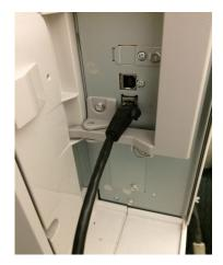
Step 9: Install CACStar I/O cover panel in place of the existing cover.
