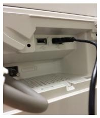
Step 6: Connect the CACStar Ethernet LAN port to your network on a port designated for this MFD.
