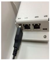
Step 5: Connect the CACStar power cable from the microUSB port on CACStar to a USB connector on the upper back of the printer.
