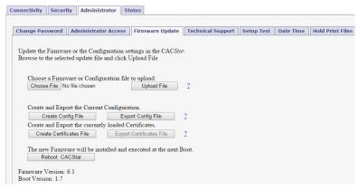
Firmware is stored in flash memory and can be updated as necessary for addition of new features. The CACStar.cfg file may also be uploaded. It
