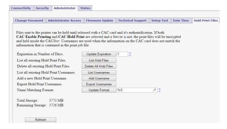
Hold Print files will be stored encrypted in CACStar and can be printed with CAC authentication at the printer.
