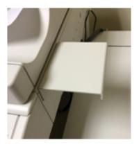
Step 2: Mount reader to top of shelf using supplied double backed adhesive preinstalled on back of reader.
